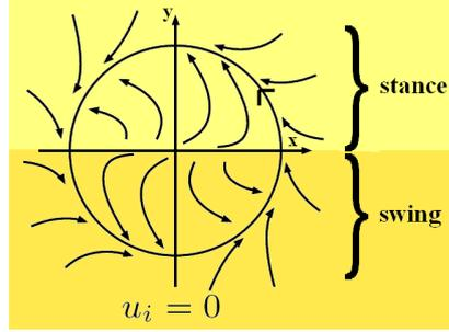
Figure 3.3: The limit cycle behavior of the CPG. If a perturbation sends point  $(x,y)$  out of the limit cycle, it would converge to it again, following the arrows.[9]
