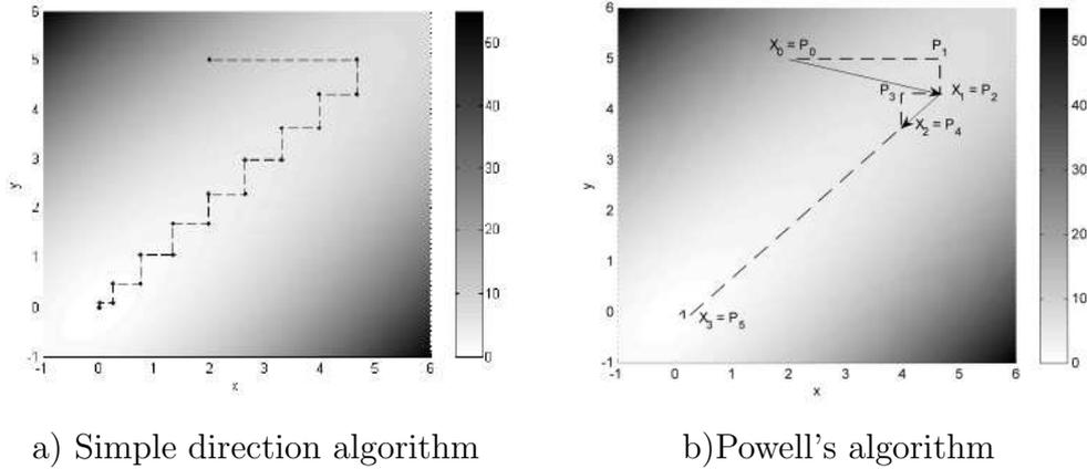
Figure 3.1: A famous example where Powell's algorithm (b) provides far better results than a classical algorithm (a). By changing the direction among which the function is minimized, Powell's reach the minimum of the function in only a few iteration, where a classical method needs about ten iterations. [6]
