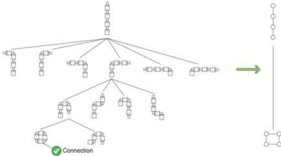
Figure 2.9: An example of the tree of all possible servo movements. Here we use this tree to find which operations leads to a square or circle architecture from a snake architecture. [4]
