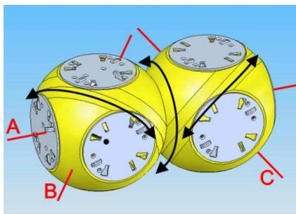
Figure 4.2: The Roombot module, with its three axes of rotation A, B and C
