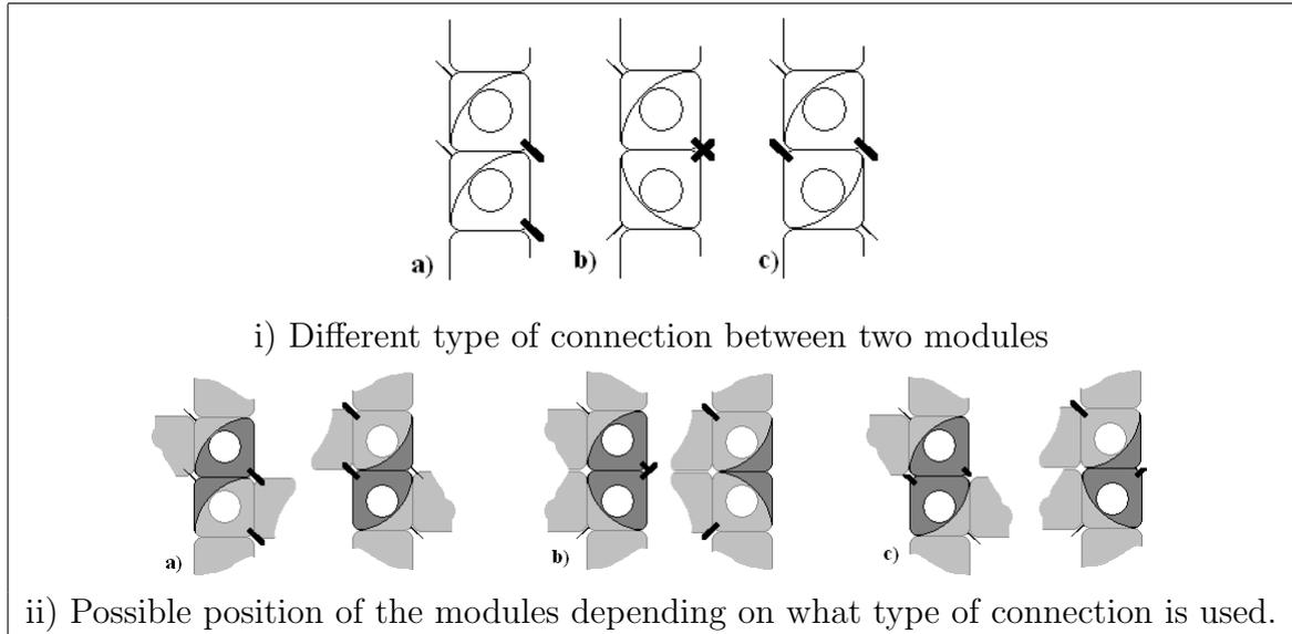
Figure 4.5: The three type of connection between two modules are parallel (a), perpendicular (b) or skew (c).
