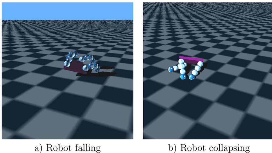
Figure 5.5: This robot's experiments show a lack of stability of the robot. If the maximal torque allowed in simulation is too high (8Nm), the robot falls. If the maximal torque allowed is too low (4Nm), the the robot can't support its own weight and collapses.
