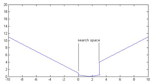
Figure 4.8: The fitness function for a limited search space is extended to an infinite search space by replacing  $f(P) = \frac{1}{1+D}$  by  $f(P) = 1 + ||P||$  if  $P$  is out of range
