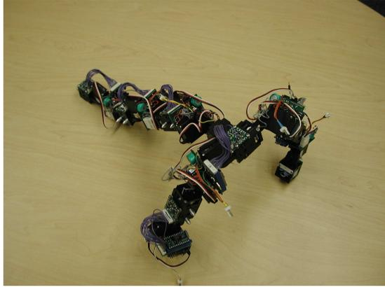
Figure 4.7: CONRO Tripod Robot: Two legs are symmetric and are used for locomotion. The third one is like the prolongment of the body and is useful because it increases the stability of the gait. [2]
