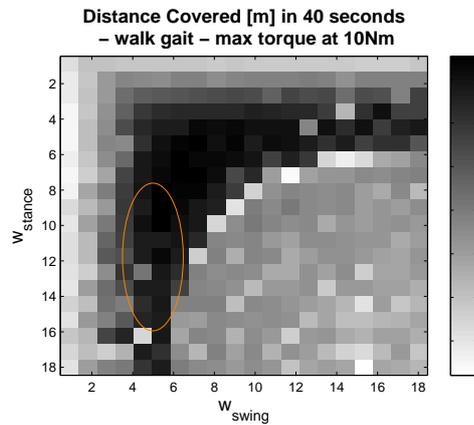
Figure 6.3: Here again, the distance covered in a simulation run seems to be dependant of both  $\omega_{swing}$  and  $\omega_{stance}$ .
