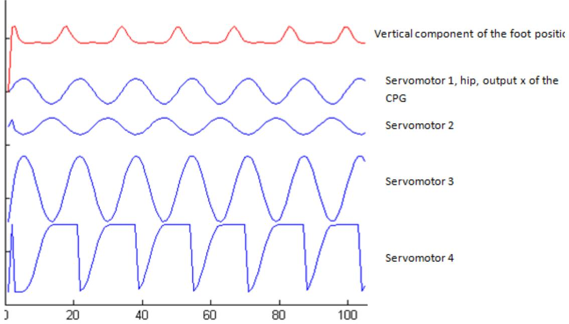
Figure 5.7: The command send to the 4 motors in blue, and the resulting vertical motion of the foot (in red) among time. The desired pattern was reached: The foot remains at the same height during half a cycle and then the leg length bends during the other half cycle.
