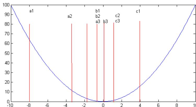
Figure 3.2: Three iteration of Golden Section Search algorithm. At each iteration, we have three points  $a_i$ ,  $b_i$  and  $c_i$ , such that  $f(b_i)$  is lower than both  $f(a_i)$  and  $f(c_i)$ .
