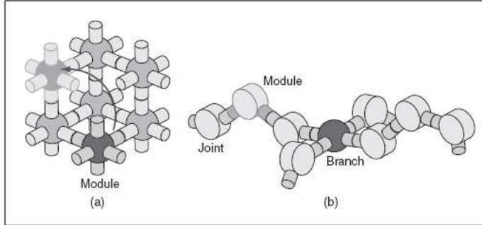
Figure 2. Types of SR robots. (a) Lattice type. (b) Chain type.
