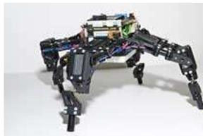
Figure 2.5: Hob Lipson's spider robot is aware of its own structure and can find new locomotion gaits if the robot's structure changes (a broken limb for example). Such behaviors are researched in modular robotics because it allows to adapt to a new robot's structure.[3]
