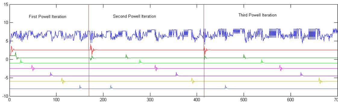
Figure 5.1: Iterations of Powell's optimization for modules that works in oscillation. The first line is the distance covered in a simulation run, the 2nd to 8th lines are the 7 open parameters. After optimization,  $D_{max} = 4.30$
