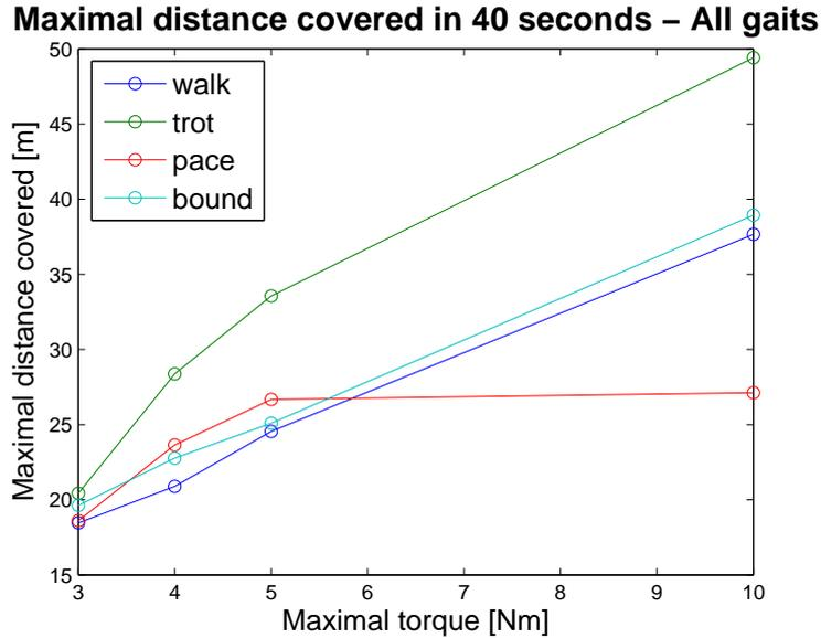
Figure 6.1: The best distance covered for each gait and different maximal torque values. Trot gaits has systematically the best results.
