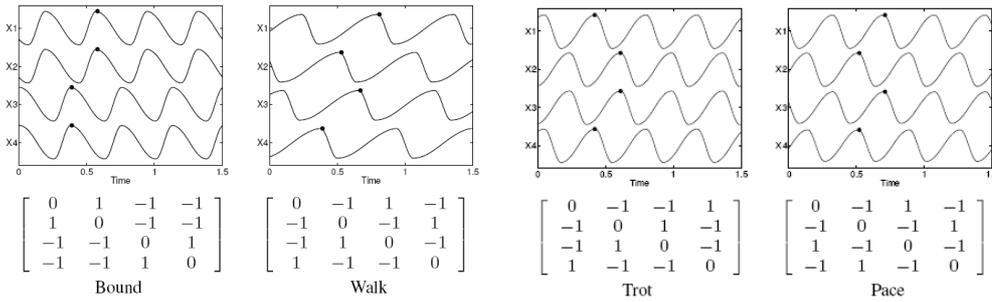
Figure 3.5: Coupling matrices and examples of gait generation for the 4 gaits.  $\omega_{stance} = 2 \cdot \omega_{swing}$  for the trot and pace gaits,  $\omega_{stance} = 4 \cdot \omega_{swing}$  for the walking gait and  $\omega_{swing} = 2 \cdot \omega_{stance}$  for the bound.[9]
