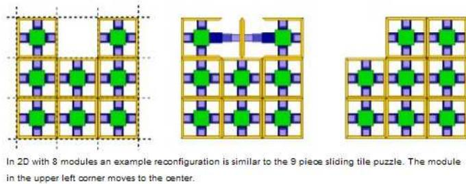
Figure 2.7: Telecube modules in a 2D reconfigurable lattice. [10]
