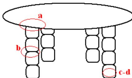
Figure 4.3: This chapter will take as an example this four-legged robot. We make the distinction between the different parameters: a) Connection between modules and passive elements, b) connection between different modules, c) servo parameters and d) CPG-model parameters.
