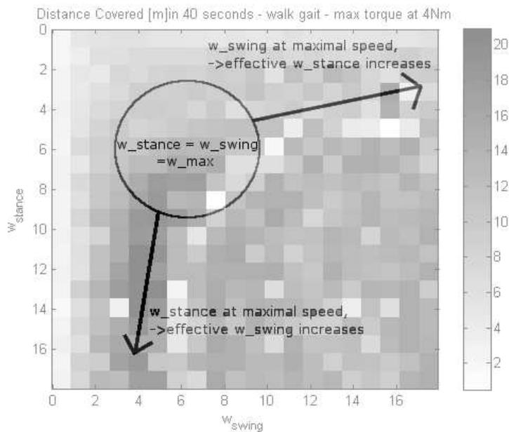
Figure 6.5: When one of the speeds reaches its maximum, the other speed increases for compensate, as illustrated.
