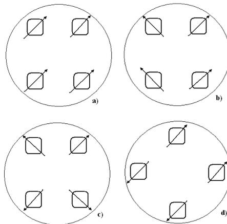
Figure 4.4: Four examples of connecting the modules to the passive element. Arrows represent the axis of rotation of the first servo motor.
