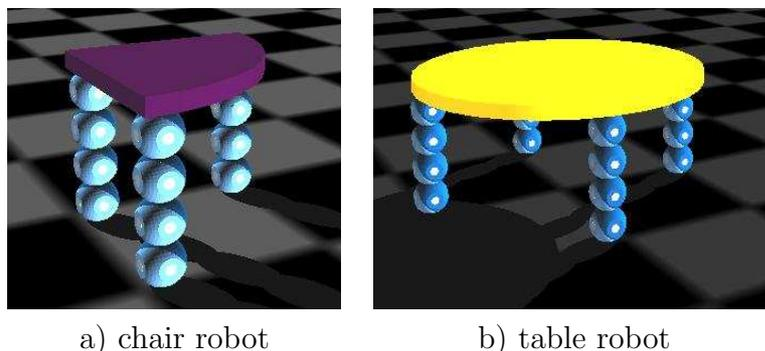
Figure 4.1: Two robots that were used for the simulations. Initially, robot a) was designed as a chair and robot b) as a table. Finally they don't have good dimensions, neither sufficient torque to be used as real pieces of furniture.
