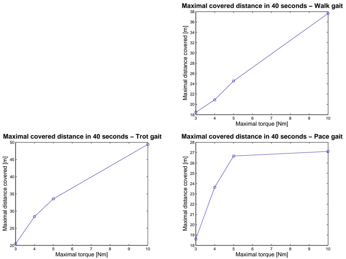
Figure 5.9: Results of systematical search for the different gaits, according to the maximum torque allowed.
