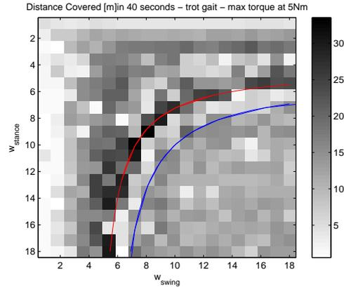
Figure 6.4: The curve of theoretical speed of saturation (in blue) and the effective curve of speed saturation (in red) don't coincide. For this trot gait at 5Nm, the theoretical maximal speed is of 5 rad/sec, but it is observed at 4.2 rad/sec.
