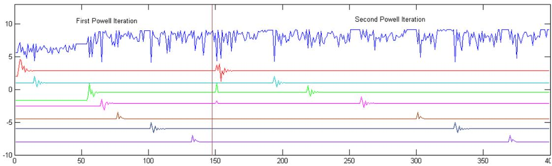
Figure 5.4: Iterations of Powell's optimization. Motors 2 and 3 works in rotation while the others are in oscillation mode. The first line is the distance covered in a simulation run, the 2nd to 8th lines are the 7 open parameters. After optimization,  $D_{max} = 5.14$
