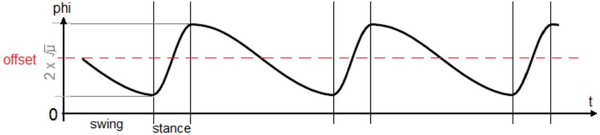
Figure 4.6: An illustration of the servomotor parameters  $\omega_{stance}$  and  $\omega_{swing}$ , offset and amplitude of the signal
