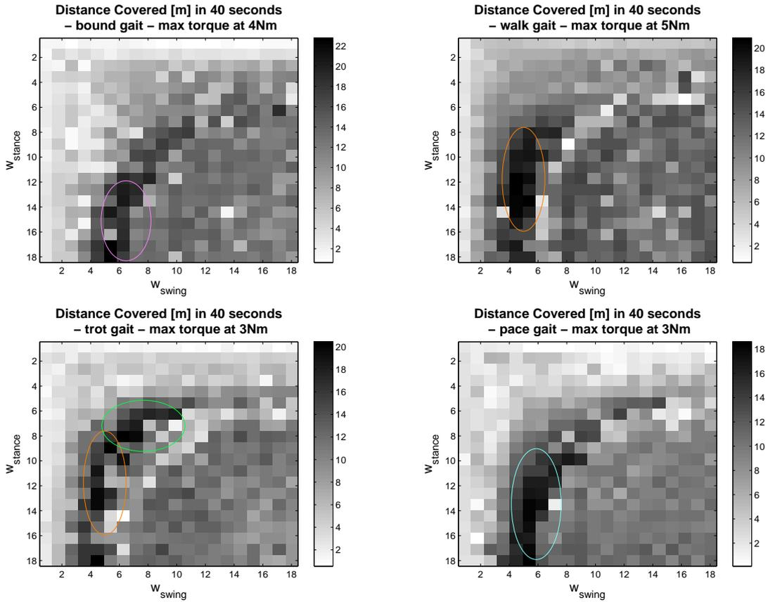
Figure 6.2: The ellipses show the areas of the search space where the distance is maximal. However, according to [9], the plots should have horizontal strips, because the speed of locomotion is not dependant of  $w_{swing}$ .
