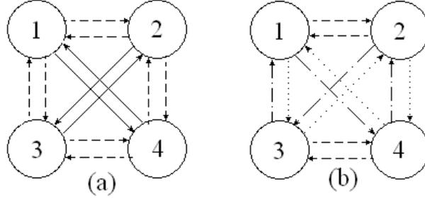
Figure 3.4: Trot gait(a) and Walk gait(b) on a quadruped animal. Each different type of arrow stand for different coupling between the legs.
