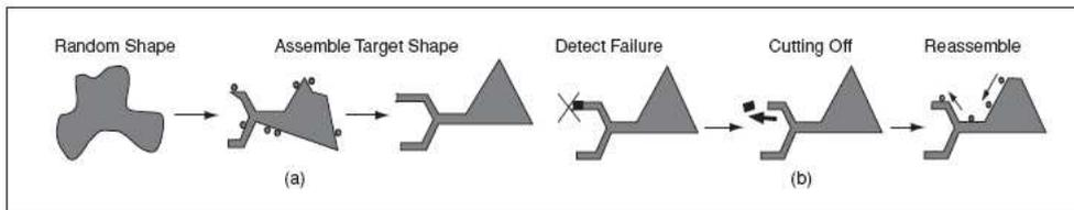
Figure 2.4: Schema of the concept of auto-assemble and regeneration in Modular Robotics. In (b), an unused part of the robot is carried to the missing part for replace it. [8]
