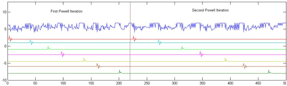
Figure 5.3: Iterations of Powell's optimization. Motor 2 works in rotation while the others are in oscillation mode. The first line is the distance covered in a simulation run, the 2nd to 8th lines are the 7 open parameters. After optimization,  $D_{max} = 2.80$
