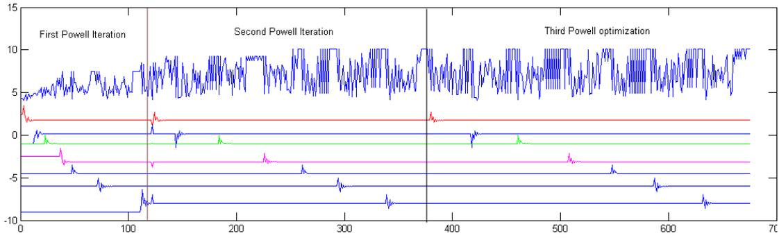
Figure 5.2: Iterations of Powell's optimization. Motor 3 works in rotation while the others are in oscillation mode. The first line is the distance covered in a simulation run, the 2nd to 8th lines are the 7 open parameters. After optimization,  $D_{max} = 6.11$
