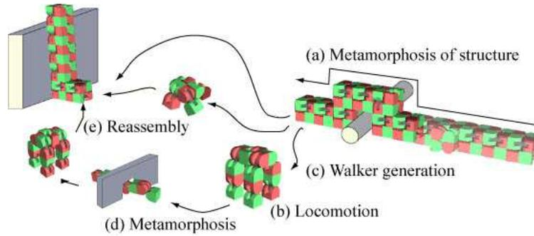
Figure 2.3: The potential of adaptability to new situations for the MTRAN modules. By reassembly, the robot can configure itself in different structures that allows climbing on obstacles, (a) and (e), locomotion (b), or taking reduced passages(d). This behaviors are inspired from the collaborative animals like the ants: little structures assemble and reassemble to make efficient robots that solve local problems. <http://unit.aist.go.jp/is/dsysd/mtran3/what.htm>
